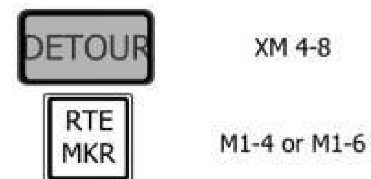
(F) BI-DIRECTIONAL CONFIRMING DETOUR ROUTE MARKER ASSEMBLY
